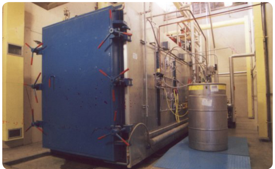
ABOVE: A typical sterilisation chambers using ethylene oxide
